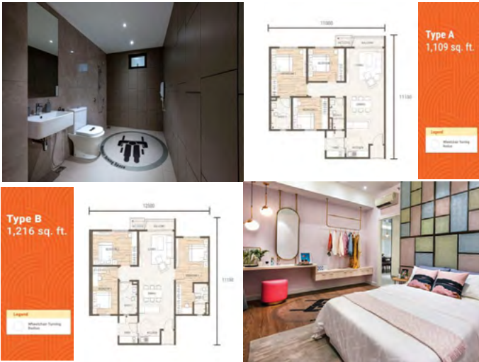
Figure 5.27: Wheelchair Turning Radius Design
