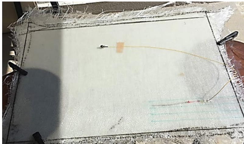
Figure 26.1: GFRP panel during the fabrication process
