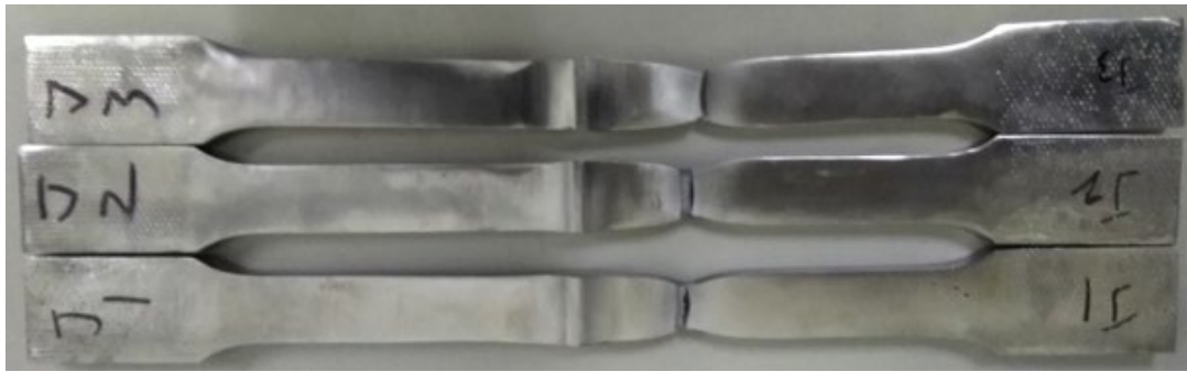
Figure 18.1: The specimen of tensile ELCC butt joints
