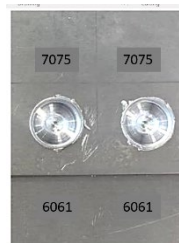
Figure 11.4: Top view weld appearance representation of a completed spot-welded sample with parameters at level 1
