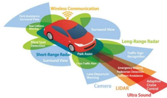
Figure 9.1: Common autopilot sensor components
